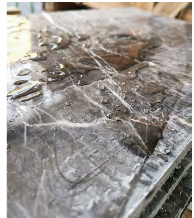
3. Water proof testing
