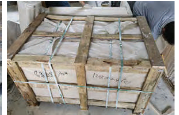
5. Nailing the cover and having a belt packing
