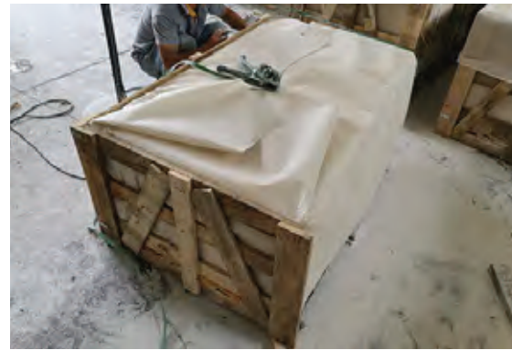
3. Covering the wooden case by foam
